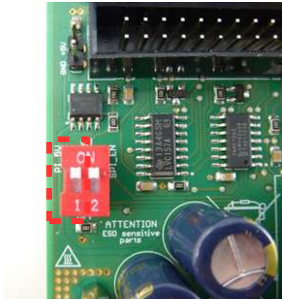
Figure 29: “PI_5V” in the “ON” position
