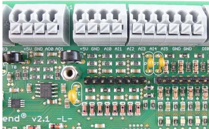
Figure 69: Terminal blocks - analog inputs and outputs
