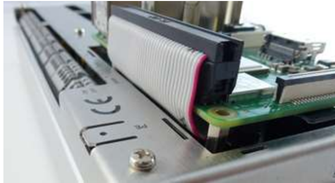
Figure 23: Optimal routing of the ribbon cable
