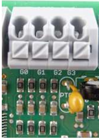
Figure 66: Terminal block connection - GPIOs
