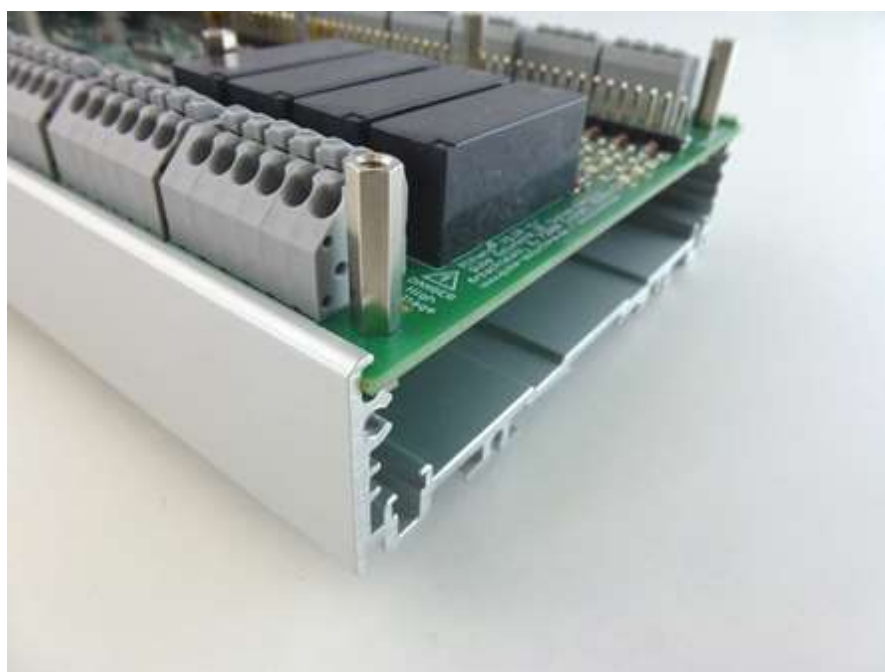
Figure 13: Connecting the PiXtend and housing profile together
